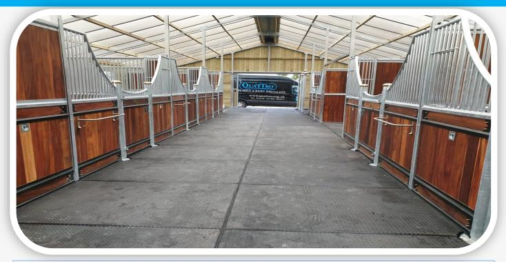
Quattro developed the Bonded & Sealed matting system over 20 years ago to alleviate the problem of urine, bedding and dirt getting under loose fitted mats which can make stables unhygienic and cause strong odours plus lifting mats in and out of stables to clean underneath is extremely difficult. The Bonded & Sealed Matting can be fitted in to Stables, Wash Boxes, Treadmills, Turn Out Pens & Walkways
